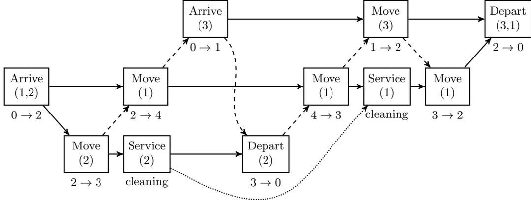
Figure 5: The partial order schedule of the shunting plan described in Section 3.1. The nodes represent train activities, with the corresponding train between parentheses, and the arcs indicate precedence relations of activities that require the same train unit (solid arcs), service resource (dotted), or movement infrastructure (dashed). The  $i \rightarrow j$  notation below a node indicates a movement from track  $i$  to track  $j$ .
