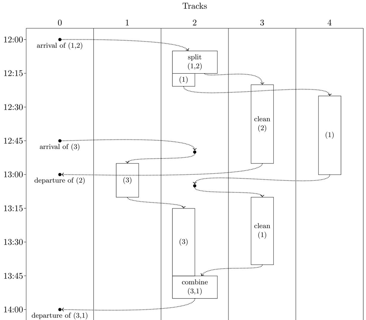
Figure 4: An overview of the positions of trains over time in the shunting plan listed in Table 3. Dotted lines represent train movements.
