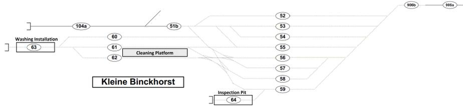
Figure 1: The “*Kleine Binckhorst*” shunting yard is operated by NS. The yard contains a washing installation at track 63, a cleaning platform between tracks 61 and 62, and an inspection pit at track 64. Tracks 52 to 59 are used to park trains. The lengths of these parking tracks range from 202 to 480 meters, and each track can contain multiple train units.
