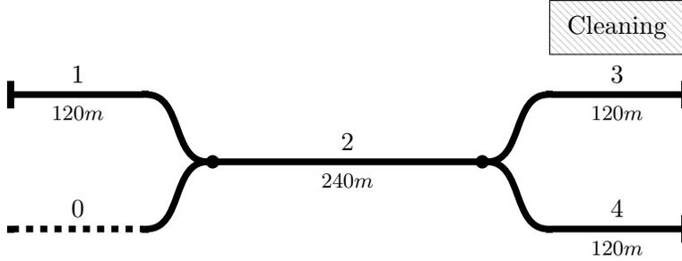
Figure 3: An example of a service site. Trains enter and exit the site over track 0 and can only be parked on tracks 1 to 4. The tracks are connected by two switches. The length of the parking tracks is displayed in meters. A cleaning platform allows internal cleaning tasks to be performed on trains positioned on track 3.
